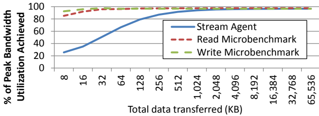
Fig. 3: Streaming double precision 64-input DFT performance and DRAM controller microbenchmark results on the DE4.
